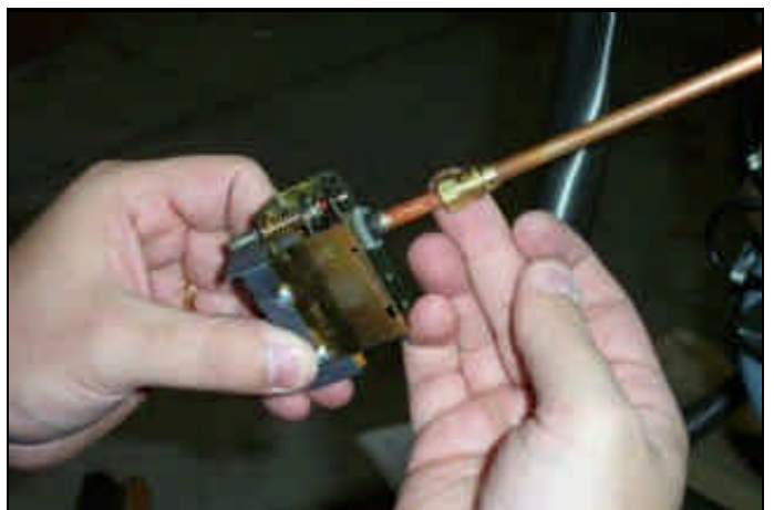
Sliding imperial fitting onto new thermostat.
